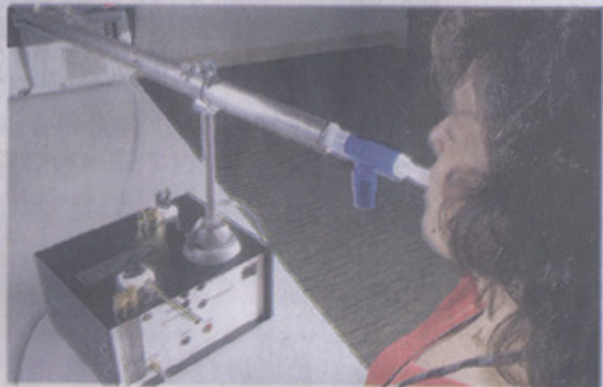
GIVING A SAMPLE: A demonstrator blows into a sensor that absorbs volatile organic compounds in the breath for later measurement.
