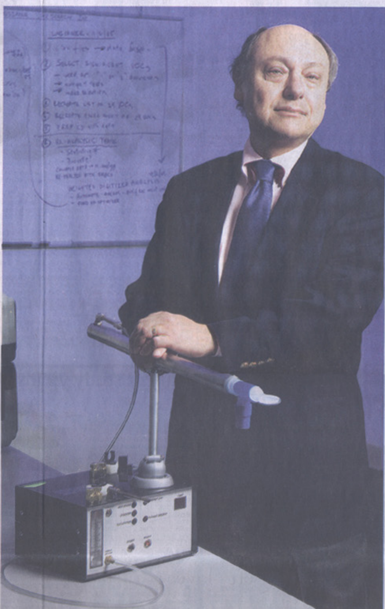
EASY AND PAINLESS: Sensors detect disease by checking for key chemicals in the breath. The device developed by Dr. Michael Phillips of New York Medical College could become the first FDA-approved method of lung cancer screening.
