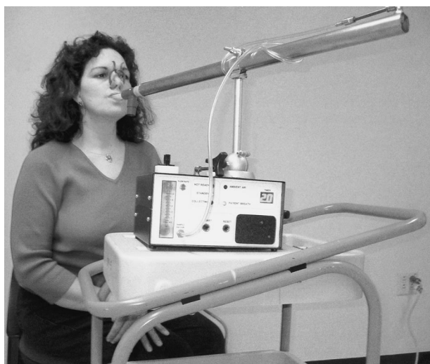
FIGURE 2. The breath collection apparatus is shown in use. The subject wears a nose clip and breathes quietly in and out through a disposable mouthpiece. The long tube is the breath reservoir, and the small tube affixed to its end is the sorber trap, which captures the VOCs in the breath. The front panel of the breath collection apparatus shows the flowmeter on the left and a digital timer on the top right.
