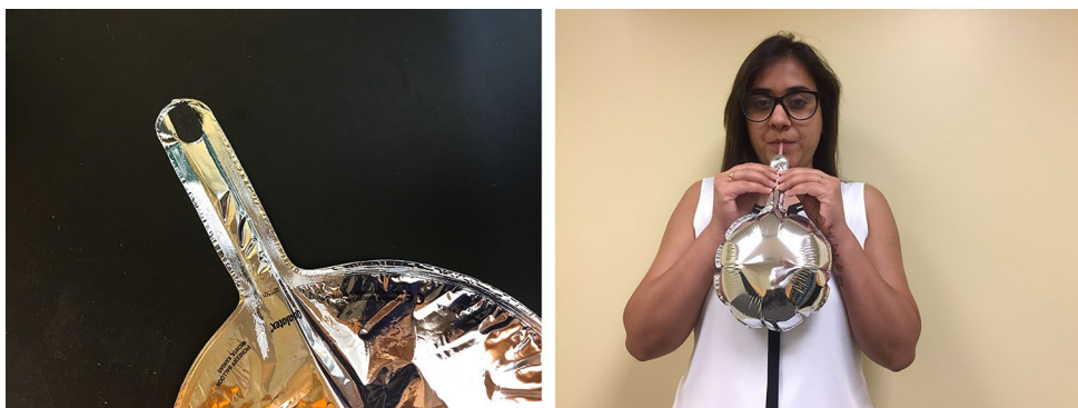
Fig. 2 Ultra-clean breath collection balloon. Balloon with activated charcoal reservoir (left hand panel): This figure shows the neck of the balloon with the indwelling reservoir, a paper strip impregnated with activated charcoal that captures >99% contaminant VOCs by sorbent trapping. The activated charcoal reservoir is removed from the
